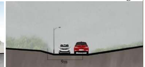
Slope degree: 3 & road with 9M
