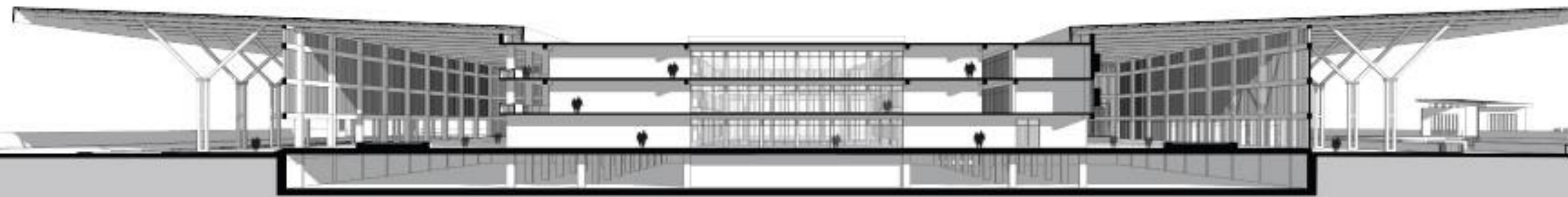
PERSPECTIVE SECTIONAL VIEW 1 This section shows the triple height arrival & departure zone with sloped roofing continued till triple height entrance foyer & waiting respectively. Both wings are connected with 9m wide walkway with view of internal & external plaza on both sides as shown in section.
