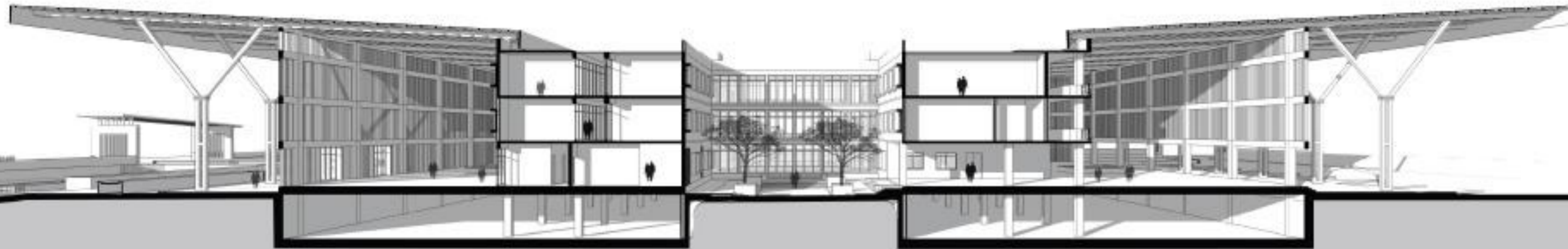
PERSPECTIVE SECTIONAL VIEW 2 This section shows the triple height arrival & departure zone with sloped roofing continued till triple height entrance foyer & waiting respectively. Central portion is open to sky courtyard with public plaza which is connected to the restaurants & walkways in elevation.
