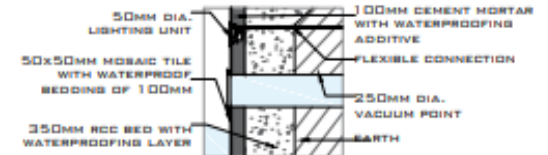
LIGHTING AND VACUUM SUCTION HOLE DETAIL AT = 1:20
